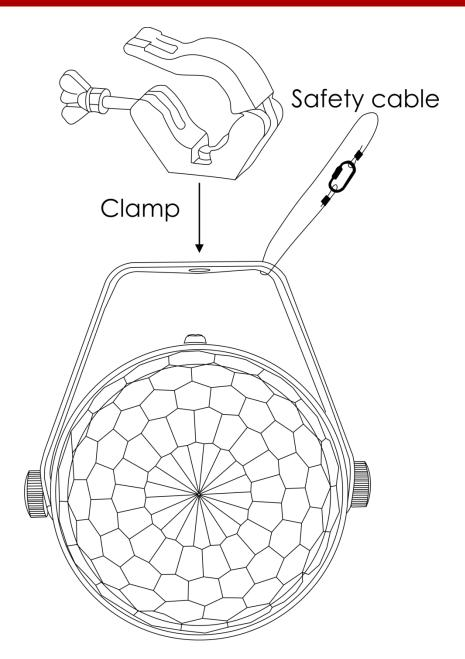
The Bumper Stars can be placed on a flat stage floor or mounted to any kind of truss with a clamp.
