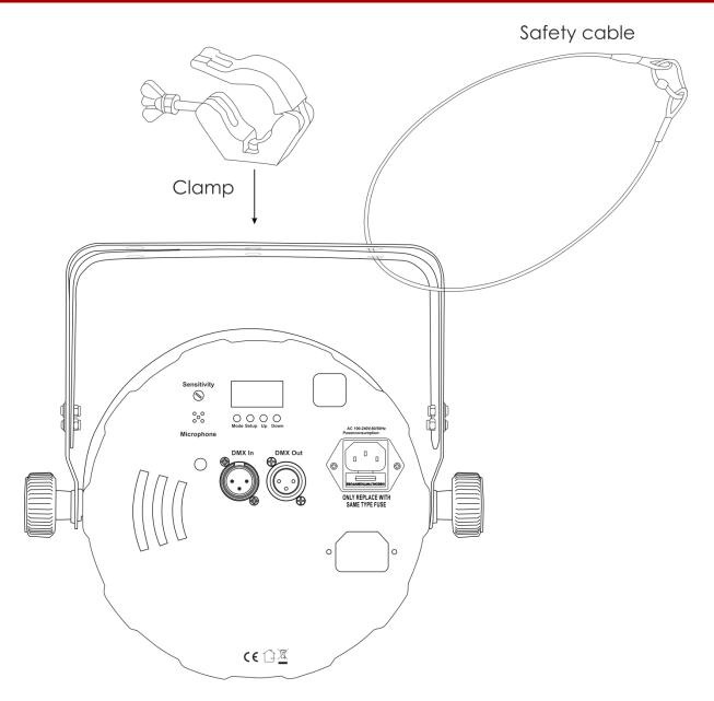
The Club Par 18-1 RGB can be placed on a flat stage floor or mounted to any kind of truss with a clamp.
