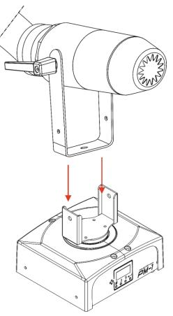
02) Insert and tighten the mounting screws (Fig. 04).
