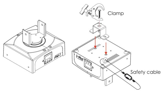
The PM-1 can be placed on a flat stage floor or mounted to any kind of truss with a clamp.
