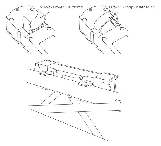
The PowerBOX 4C can be placed on a flat stage floor or attached to any kind of truss, with the **90659** – PowerBOX clamp or the **D9575B** – Snap Fastener 22.
