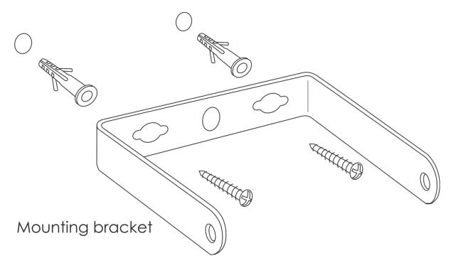
The Floodlight can be placed on a flat stage floor or mounted to a wall.
