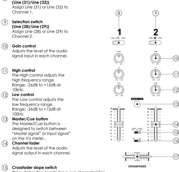
This switches the crossfader curve characteristics.
