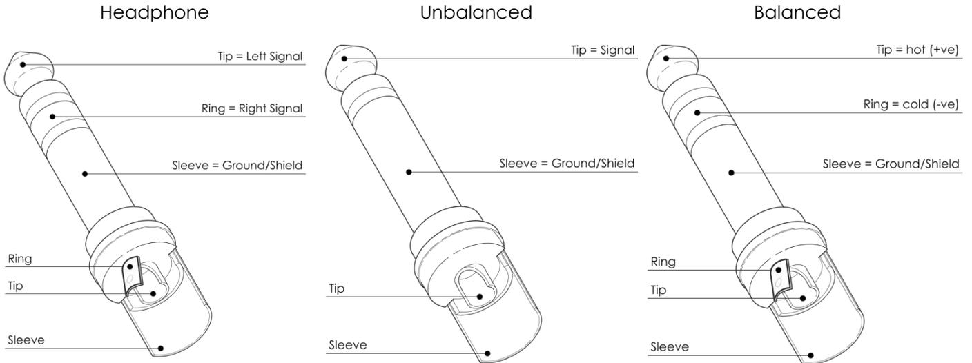
For these applications the unit provides 1/4" TRS and XLR connectors to easily interface with most professional audio devices. Follow the configuration examples below for your particular connection.
