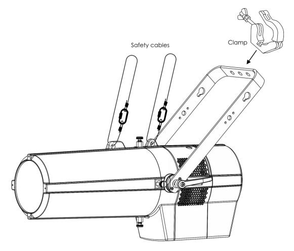
The Performer can be mounted to any kind of truss with a clamp.
