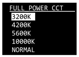
01) Press the **UP/DOWN** buttons to choose the desired color temperature. The available options are: 3200K, 4200K, 5600, 10000K and NORMAL.
