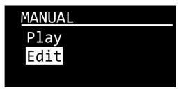
01) Press the **UP/DOWN** buttons to choose EDIT and press the **ENTER** button to open the menu. The display will show:
