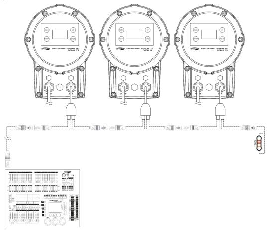
Note: Link all cables before connecting electric power
