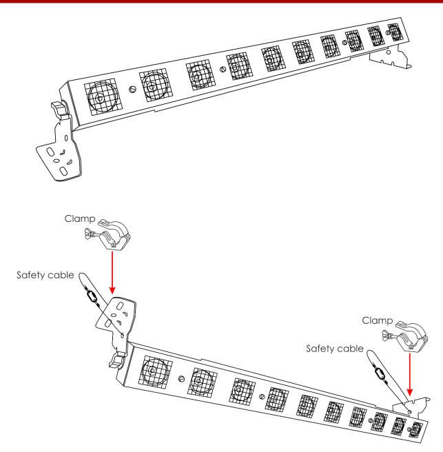
The Sunstrip Active MKII 110V can be placed on a flat stage floor or mounted to any kind of truss with a clamp.
