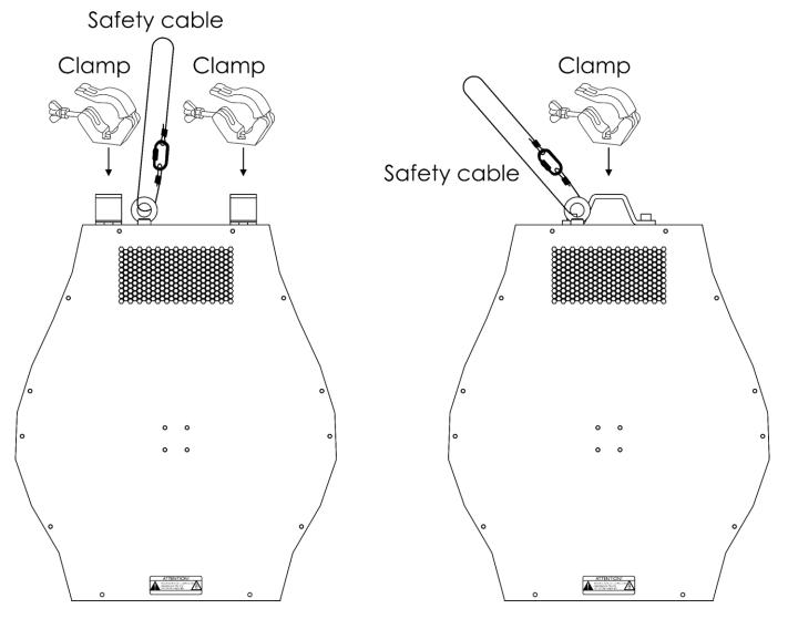
The Illumilift can be mounted to any kind of truss with 1 or 2 clamps.
