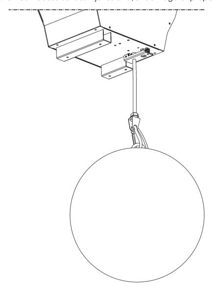
The Illumilift LED Sphere can be mounted to the Illumilift RGBW (41165) or the Illumilift RGBW Turbo (41166).
