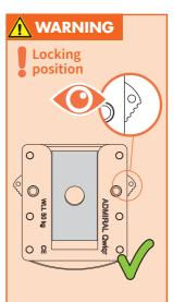
If you see the dots on both locking switches, the Qwigr is locked.
