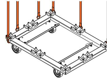
secure with sufficient lashing straps
