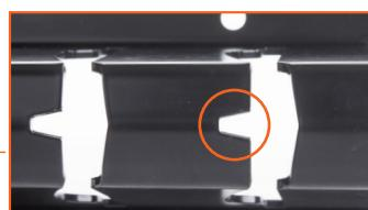
Indicator indicates which side the conical couplers should be.
