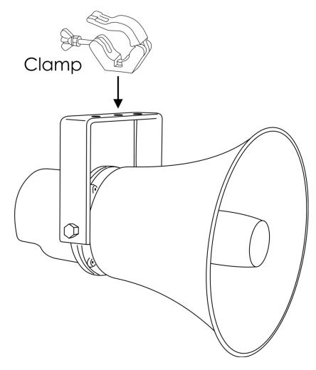
The HS-30R can be mounted to any kind of truss with a clamp.
