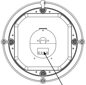
Connect the main feed cable (+) and the common cable (-)
