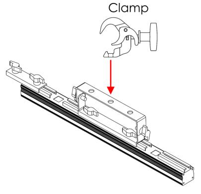
The Pixelstrip 20 can be mounted to any kind of truss with a clamp.
