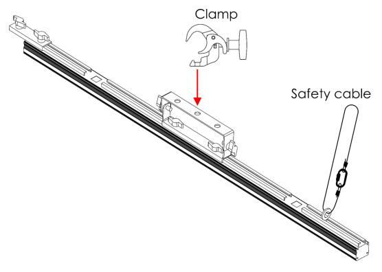
The Pixelstrip 40 can be mounted to any kind of truss with a clamp.
