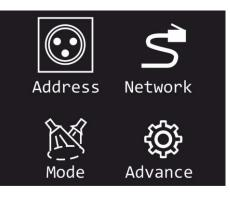
**Note:** If no button is pressed, after 20 seconds of inactivity the display will return to the start screen and after 10 more seconds it will turn off. Press any button to turn the display on.
