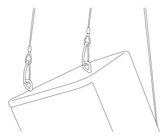
The Pure-15 speaker can be placed on a flat stage floor or be hung from a ceiling by means of the Speaker hanging eye (D8436).
