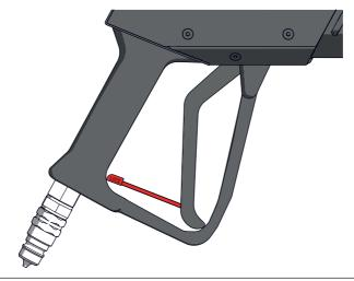
Connect the CO<sub>2</sub> hose to the CO<sub>2</sub> quick connector.
