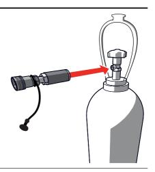
Connect the CO<sub>2</sub> hose to the CO<sub>2</sub> Bottle to Hose Connector on the CO<sub>2</sub> cylinder.
