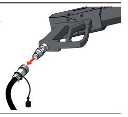
Disconnect the CO<sub>2</sub> hose from the CO<sub>2</sub> Bottle to Hose Connector on the CO<sub>2</sub> cylinder.
