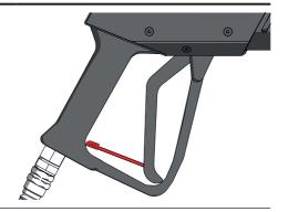
Disconnect the CO<sub>2</sub> hose from the CO<sub>2</sub> quick connector on the pistol.
