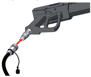
3 Connect the CO<sub>2</sub> Bottle to Hose Connector to a CO<sub>2</sub> cylinder.
