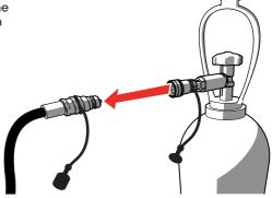
Remove the CO<sub>2</sub> Bottle to Hose Connector from the cylinder.
