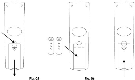
Note: Make sure that you install the batteries with correct polarity orientation.
