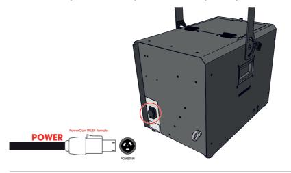
3 Connect the other end of the powerCON TRUE1 cable to the controller or power switch.
