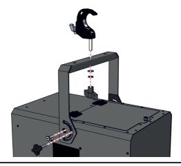
2 Mount the twenty clamp on a truss and secure with a certified safety cable.
