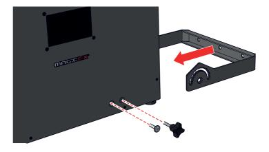
3 Place the MAGICFX<sup>®</sup> CLUBBLOWER under an angle by rotating the bracket to the bottom side of the machine and tighten the star knobs on both sides.
