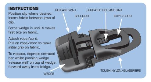
**IMPORTANT** – In the interest of maximum safety and security, the clip is designed to have exceptional gripping power; clip grip increases as the load applied increases. To ease the dismounting of the clip after heavy loading, please follow the instructions below.
