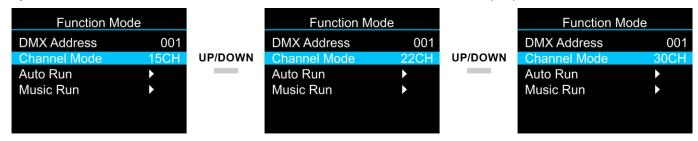
02) Press the ENTER button to confirm the desired Channel Mode.
